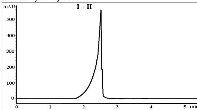
Figure 1. Chromatogram of benzoic acid (I) and potassium sorbate (II) obtained on Hypersil ODS (25 cm x 0.46 cm; 5 µm) column; mobile phase acetonitrile/water 80/20 (V/V), flow rate 1 mL/min, column temperature 25 °C and UV detection at 220 nm.
