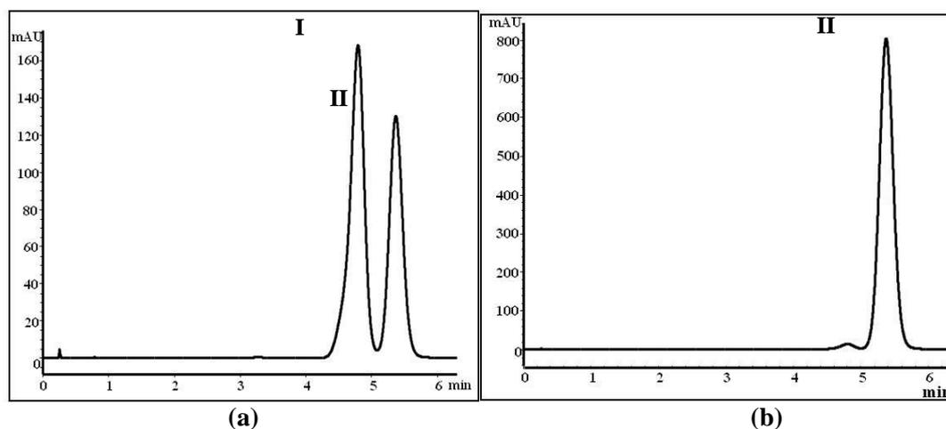
Figure 3. Chromatogram of benzoic acid (I) and potassium sorbate (II) obtained on HS (High Speed) type LiChroCART<sup>®</sup> 30-4 HPLC-Cartridge Purospher<sup>®</sup> STAR RP-18 (30 mm x 4 mm; 3  $\mu$ m) column; mobile phase methanol/phosphate buffer (pH 3.70) 20/80 (V/V), flow rate 1 mL/min, column temperature 25  $^{\circ}$ C and UV detection at 225.4 nm (a) and 255.4 nm (b).
