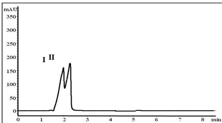
Figure 2. Chromatogram of benzoic acid (I) and potassium sorbate (II) obtained on LiChrospher 60 RP-select B (12.5 cm x 0.4 cm; 5  $\mu$ m) column; mobile phase acetonitrile/water 50/50 (V/V), flow rate 1 mL/min, column temperature 25  $^{\circ}$ C and UV detection at 220 nm.
