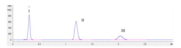
Figure 3. Chromatogram obtained on Purospher<sup>®</sup> Star RP-18 endcapped (3 cm × 4 mm; 3 μm) column from a standard mixture containing methomyl (I), methidathion (II) and propiconazole (III); mobile phase acetonitrile/water 50/50 (*V/V*), flow1 mL/min, temperature 25 °C and UV detection at 220 nm
