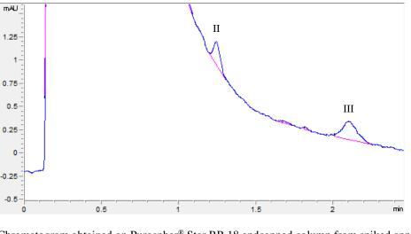
Figure 5. Chromatogram obtained on Purospher<sup>®</sup> Star RP-18 endcapped column from spiked apple juice; methidathion (II) and propiconazole (III); mobile phase acetonitrile/water 50/50 (V/V), flow 1 mL/min, temperature 25 °C and UV detection at 220 nm
