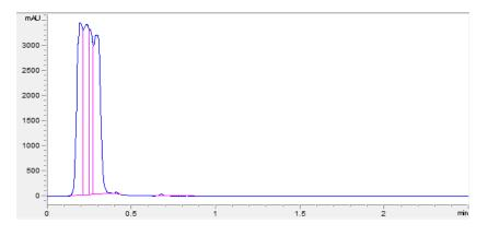
Figure 4. Chromatogram obtained on Purospher<sup>®</sup> Star RP-18 endcapped column from apple juice; mobile phase acetonitrile/water 50/50 (*V/V*), flow1 mL/min, temperature 25 °C and UV detection at 220 nm
